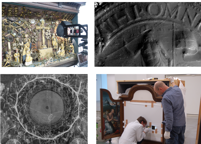
Fig.3: A-B: Microdome for digitizing with omnidirectional lighting and export to 2D+, topography of wax Agnus Dei (© Lieve Watteeuw & RICH, KU Leuven) C. RX-Imaging: Wax "Agnus Dei" attached with metal threads on a leather-textile medaillon (© KIK, Brussel, Rrx006371) D. Preventive actions for transport of the Enclosed Garden (© Willemien, Anaf, UA & KIK)
